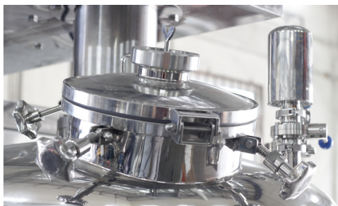
Figure 4 : Observation glass at manhole (left) comes with wiper to ensure clear view of inner tank condition while the pressure relief valve (right) is designed with safety cap.
