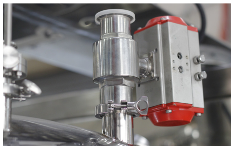
Figure 5 : Such pneumatic control valve can be opened and closed with just a touch on control panel.
