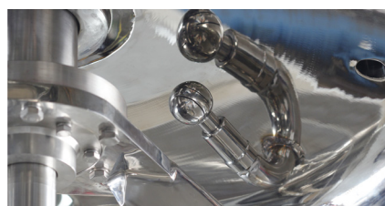
Figure 6 : Spray ball for CIP cleaning
