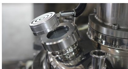
Figure 5 : LED light for observation glass/manhole
