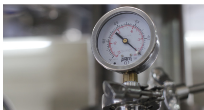
Figure 3 : Vacuum gauge for vacuum mixing
